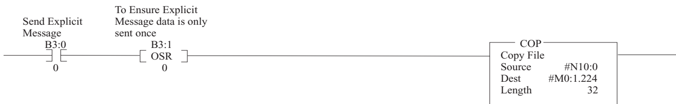
Figure C.27 Clear the DeviceNet Scanner's Response Buffer
