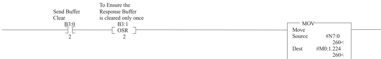
Figure C.35 Clear the DeviceNet Scanner's Response Buffer
