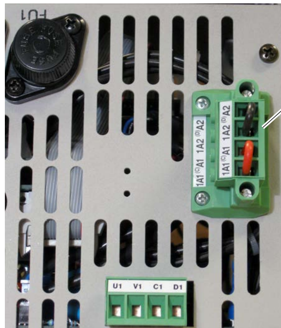
Figure 48 - PowerFlex DC - Frame B Armature Voltage Feedback Circuit Terminal Block Location
