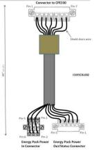
The ACC402 Energy Pack is used exclusively with the CPE330 RX3i CPU. It preserves user memory in the Controller during power fluctuations or outages.
