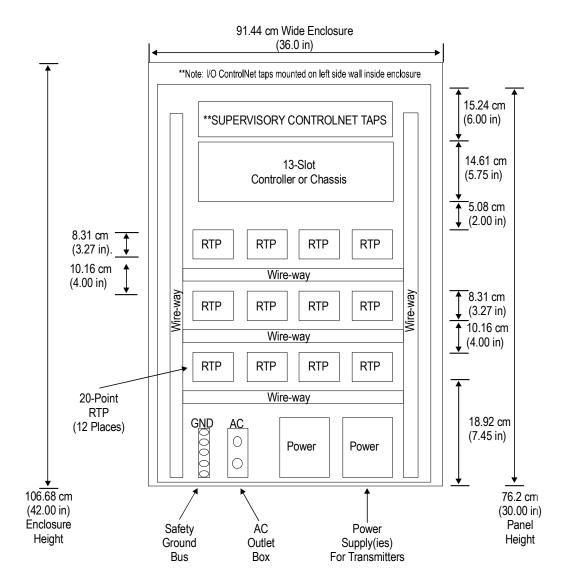
Small-scale system enclosure configuration example
