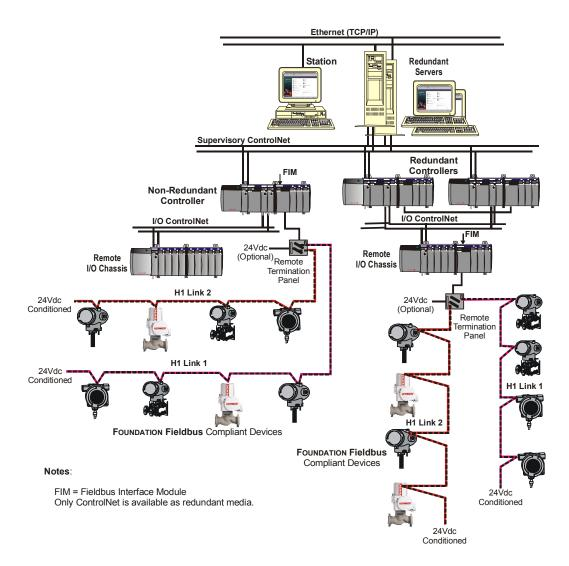
The following figure shows a typical topology using I/O Link Interface Modules to interface with Process Manager I/O.
