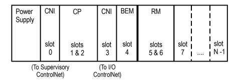
Default Module Placement for 10 and 17-slot redundant controller chassis (N = 10 or 17)
