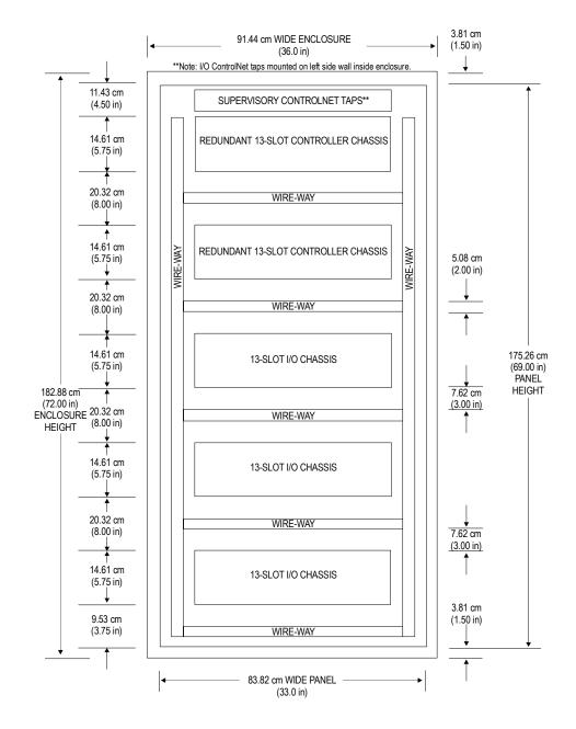
Large-scale system enclosure configuration example, 1-of-2
