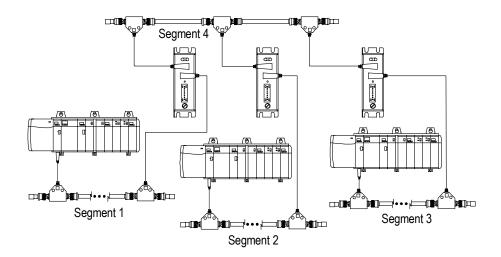
Repeaters installed in parallel
