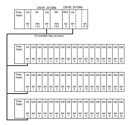
Slot numbers are labeled on the chassis' motherboard as zero through N-1; for example, zero through 12 for a 13-slot chassis. Table 2 defines the slot module defaults in this chassis.
