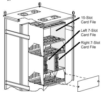
Typical 7-Slot and 15-Slot Card File Installation
