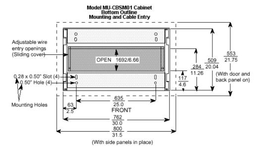
Foot print \$\improx\$ 800 x 572 mm/31.5 x 22.5 " (External dimensions - door and panels installed)
