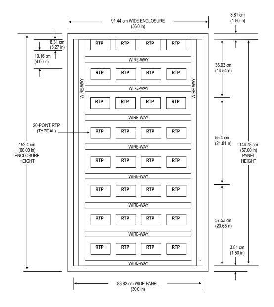
Medium-scale system enclosure configuration example, 2-of-2
