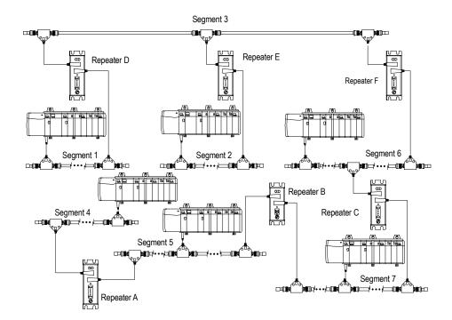
Repeaters installed in a series/parallel combination
