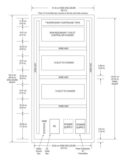
Medium-scale system enclosure configuration example, 1-of-2
