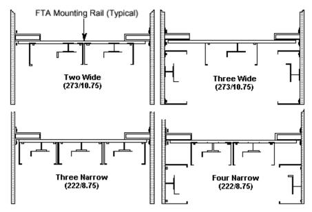
Note: Space between adjacently mounted channels is typically 6 mm (0.25 in). Dimensions are in millimeters/inches
