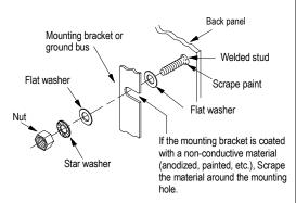
Stud mounting of a ground bus or chassis to the back panel
