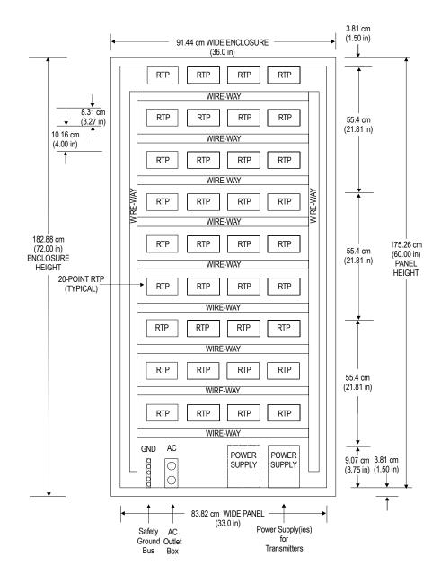
Large-scale system enclosure configuration example, 2-of-2
