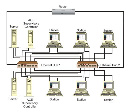
The following figure shows an alternative to the router isolation method shown above through the use of virtual networking or VLANs. You could setup a Business Network VLAN and a Plant Information Network VLAN located within the same physical hub, but yet still be physically isolated. You can make further setup of VLANs in combination with TCP/IP Subnetting to physically separate the two ethernet segments, so you do not require the use of two router port separated subnets.
