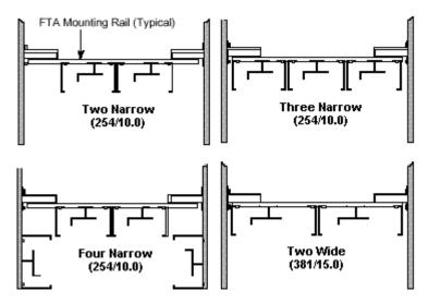
Note: Dimensions are in millimeters/inches.
