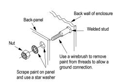
Stud mounting of the back panel to the enclosure back wall.
