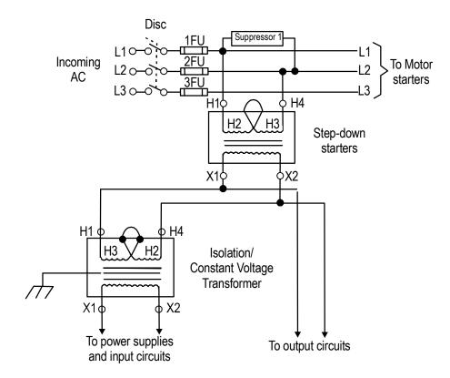
Second transformer in a power distribution system
