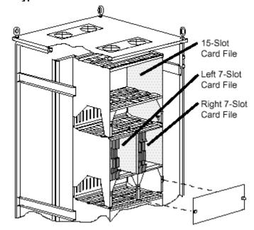
Typical 7-Slot and 15-Slot Card File Installation
