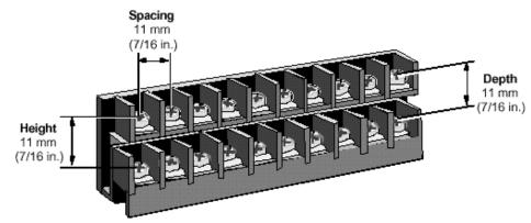
Fixed-Screw Terminal Connector for Standard Type FTA
