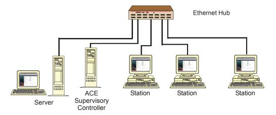
The following figure shows the topology for a Dual Ethernet option. Each Ethernet hub represents one TCP/IP subnet. The minimum Ethernet hub requirement is two separate 10 Mb/s shared hubs, although two 10/100 Mb/s switches are recommended. Note that Server redundancy is not linked to Network redundancy.
