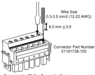
Compression Mating Connector for Galvanically Isolated Type FTA
