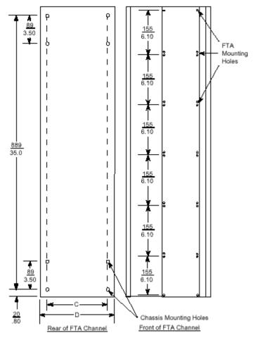
Note: See the previous figure for C and D dimensions. Dimensions are in millimeters/inches.
