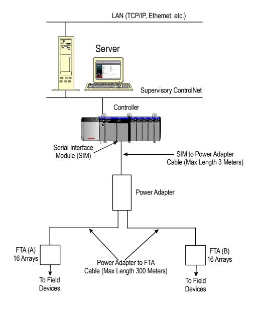
There are few restrictions to Serial Interface Module (SIM) placement. The restrictions (and recommendations) that do apply are as follows.
