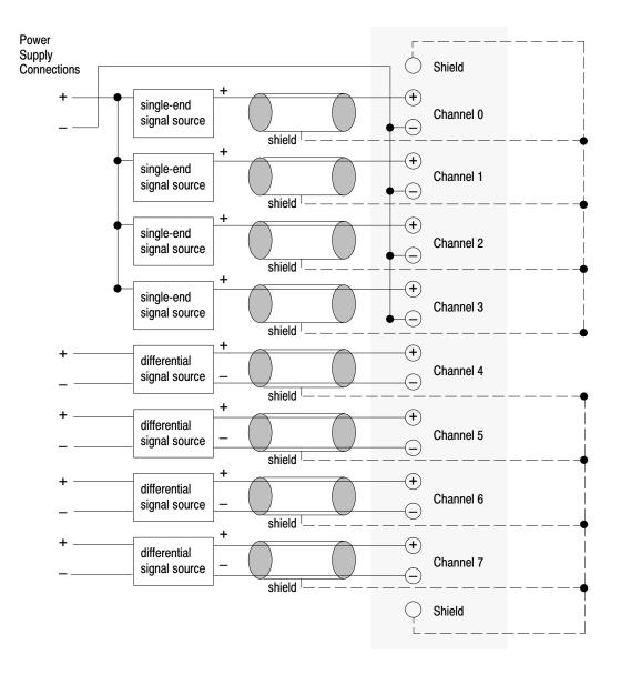
When wiring single-ended analog input devices to the analog input module, the number of total wires necessary can be limited by jumpering all "IN-" terminals together. Note that differential inputs are more immune to noise than single-ended inputs.
