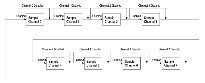
The following table shows the module update time. The module update time is the same regardless of the filter frequency. The fastest module update time occurs when only one channel is enabled. The slowest module update time occurs when 8 channels are enabled.
