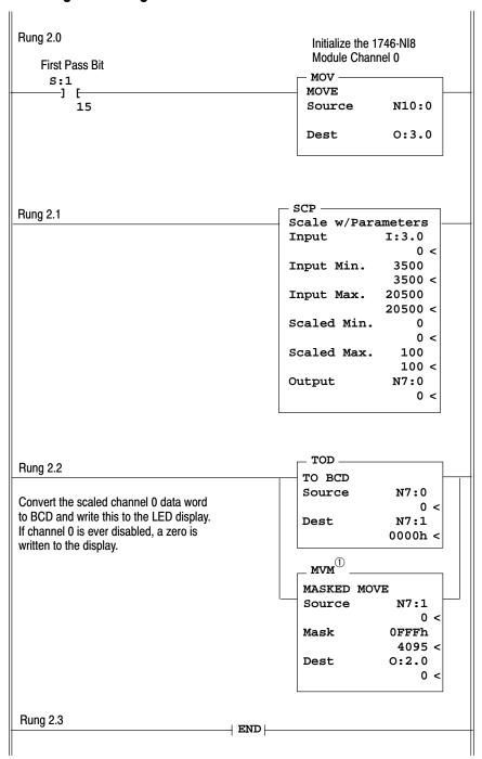
The use of the masked move instruction with the 0FFF mask allows you to use outputs 12, 13, 14, and 15 for other output devices in your system. The 7-segment display uses outputs 0–11.
