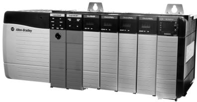
A GuardLogix® controller is a ControlLogix controller that also provides safety control. The GuardLogix system is a dual controller solution—you must use a 1756-L6xS/1756-L7xS primary controller and a 1756-LSP/1756-L7SP safety partner to achieve up to SIL CL 3/PLe/Cat. 4. A major benefit of this system is that it's still a single project, safety and standard together. The safety partner controller is a part of the system, is automatically configured, and requires no user setup.
