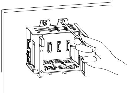
4. Leaving far-left and far-right tabs open for grounding, install the remaining tab hardware (for a four-slot chassis, leave both tabs open).
