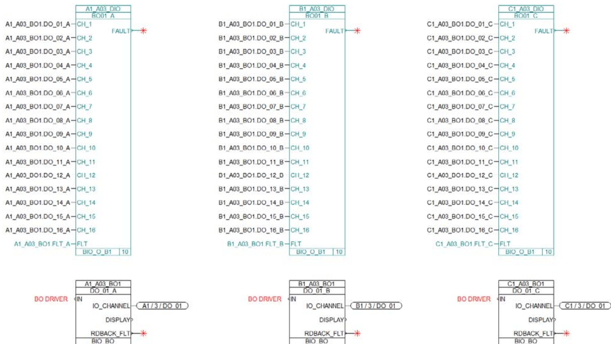
Figure 3-13. MicroNet TMR Boolean (Relay) Output GAP Configuration
