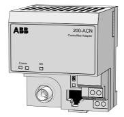
200-ACN is a remote I/O adapter unit, intended for connection of up to eight terminal base units equipped with I/O units of type S200 I/O or S200L I/O. 200-ACN is connected to the 200-CICN unit in the Advant Controller 250 via ControlNet.
