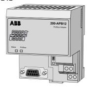
200-APB12 is a remote I/O adapter unit, intended for connection of up to eight terminal base units equipped with I/O units of type S200 I/O or S200L I/O to a Controller via a PROFIBUS-DP network.
