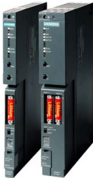
SIMATIC S7-400, POWERSUPPLY PS 405: 4A, 24/48/60V DC, 5V DC/4A, ATEXAPPROBATIONIDENTIFICATION
