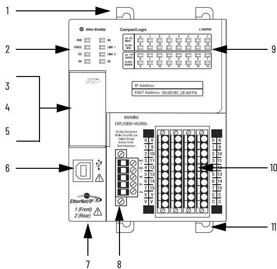
CompactLogix 5370 L1 Controller Parts
