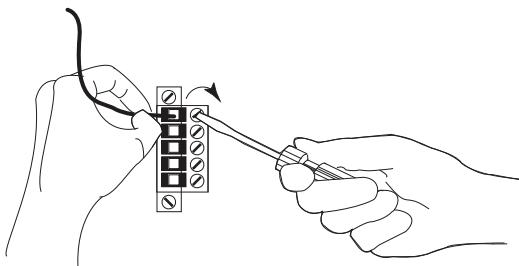
6. Connect the wire that is connected to the 24V DC- terminal on the external 24V DC power source to the VDC- terminal. The VDC- terminal is the second from the top on the removable connector.
