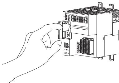
If you feel resistance when inserting the SD card, pull it out and change the orientation.
