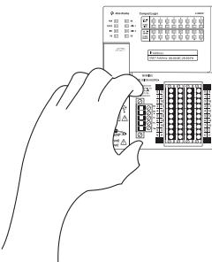
5. Connect the wire that is connected to the 24V DC+ terminal on the external 24V DC power source to the VDC+ terminal. The VDC+ terminal is the top terminal on the removable connector.
