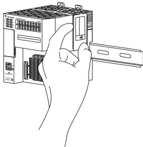
The covering covers the exposed interconnections on the right side of the controller. Failure to use a protective covering can result in equipment damage or injury from electric shock.
