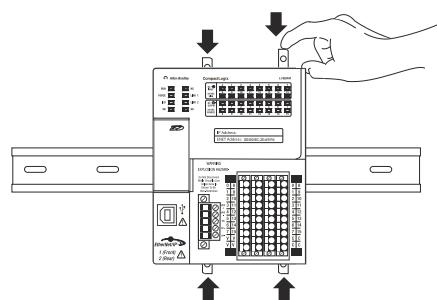
3. If you are not using local expansion modules, use the tongue-and-groove slots on the right side of the controller to slide a protective covering onto the controller.
