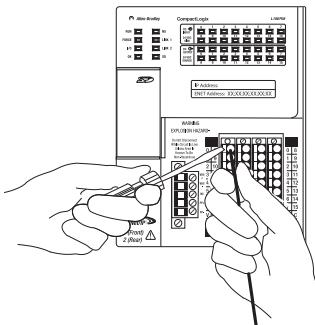
3. With the wire in place, pull the screwdriver off the spring release clip.
