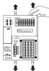
2. Slide the controller into position on the DIN rail and push the locking tabs in.
