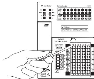
3. Pull the connector out from the I/O module to remove it.
