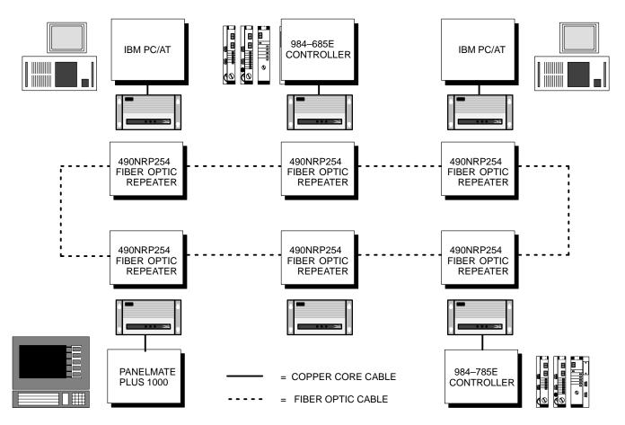
Figure 5 Example of Self–Healing Ring Configuration
