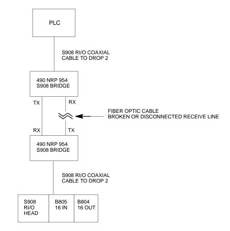
A break in the receive line as shown above will deprive the PLC of input data. Under ordinary circumstances, the PLC will continue to drive outputs via the intact transmit line. This could lead to outputs turning ON or OFF due to invalid (INPUT STATE: 0) input data.
