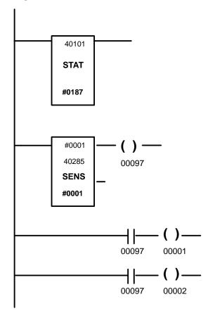
The STAT and SENS blocks monitor the I/O status of Drop #2 and inhibit outputs 00001 and 00002 if communications are lost. The STAT block provides access to the system's status, including the status of S908 communications. The status information is stored in a table which starts at 40101 and has a length of 187 words (as shown in the top and bottom nodes of the STAT block).
