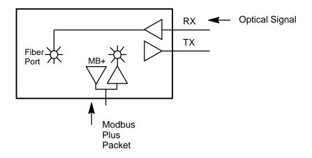
The following example makes use of this information in bringing up two point-to-point fiber optic repeaters. Connect the repeaters as shown:
