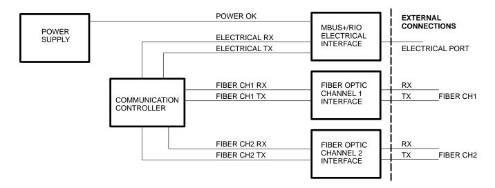
Figure 1 Simplified Internal Schematic of Fiber Optic Repeaters
