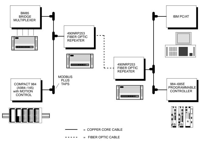
Figure 2 Example of Point-to-Point Connection
