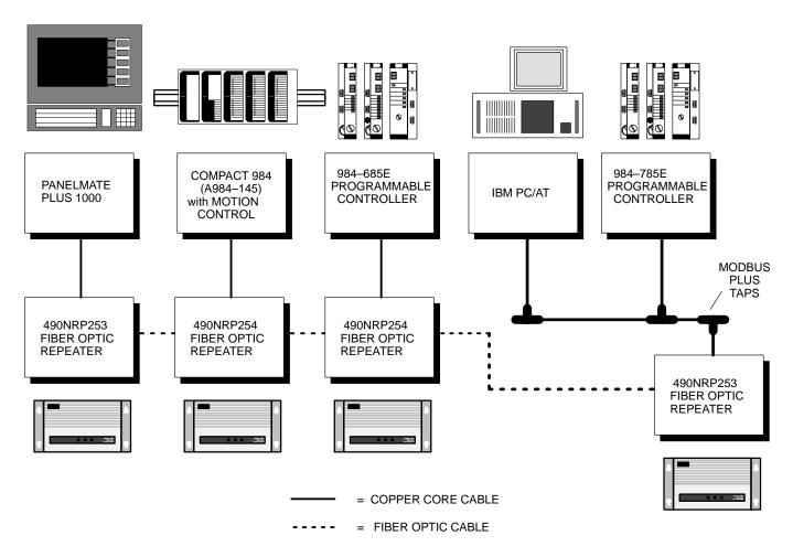
Figure 3 Example of Repeaters in a Bus Configuration
