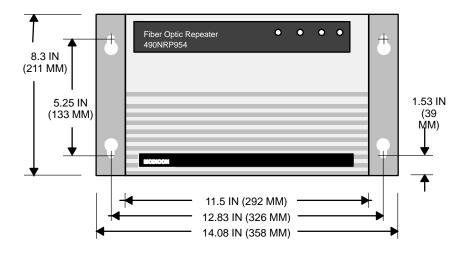
ALLOW 4.0 IN (100 MM) REAR CLEARANCE FOR ACCESS TO SWITCHES, CABLES, AND FUSE
