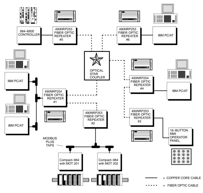
Figure 4 Example of Optical Star Configuration
