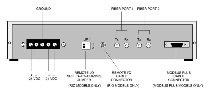
Figure 8 Rear Panel Connectors
