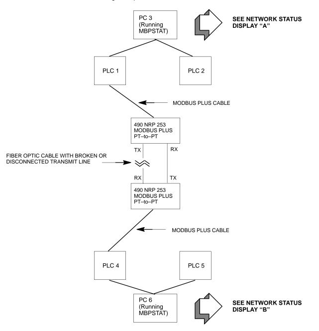
Note that the sample network consists of six nodes, three on either side of each Fiber Optic Repeater.
