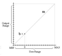
The gain, m, and offset, b, coefficients are calculated as follows:
