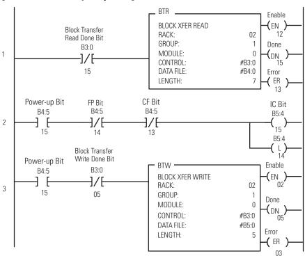
Figure 3.12 PLC-3 Family Sample Program Structure for a 1794-IF2XOF2I Module
