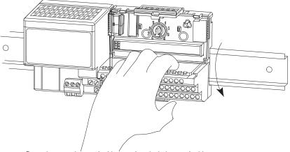
Press down on the terminal base unit to lock the terminal base on the DIN rail. If the terminal base does not lock into place, use a screwdriver or similar device to open the locking tab, press down on the terminal base until flush with the DIN rail and release the locking tab to lock the base in place.
