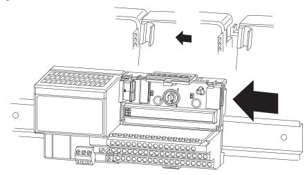
Slide the terminal base unit over tight against the adapter. Make sure the hook on the terminal base slides under the edge of the adapter and the flexbus connector is fully retracted.
