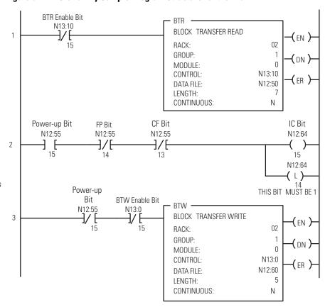
Figure 3.15 PLC-5 Family Sample Program Structure for the 1794-IF4I
