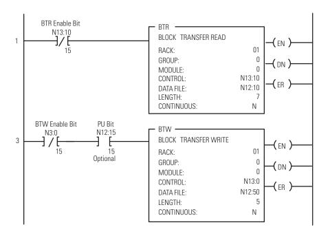
An XIC (--) [--) instruction of the Power Up bit (PU) can be inserted to allow BTWs only when the module requires configuration (PU = 1).
