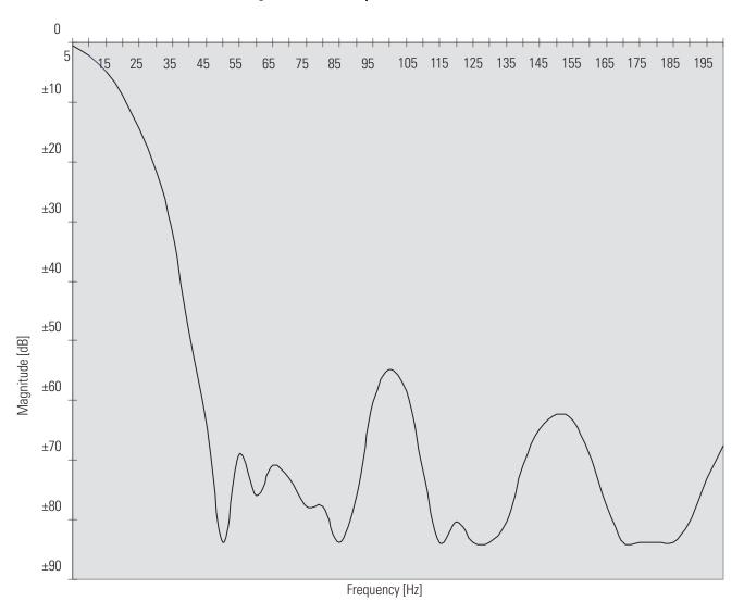
Figure A.3 Filter Response at 600 Hz Conversion
