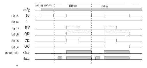
Figure 7.3 Output Calibration Timing Diagram
