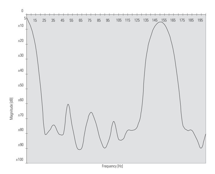
Figure A.2 Filter Response at 300 Hz Conversion
