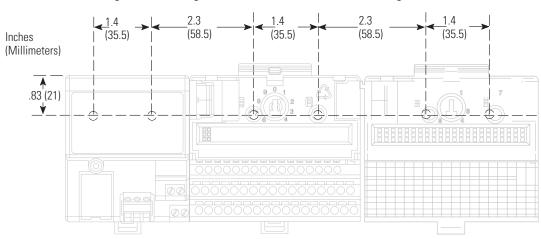
Figure 2.6 Drilling Dimensions for Panel/Wall Mounting of FLEX I/O
