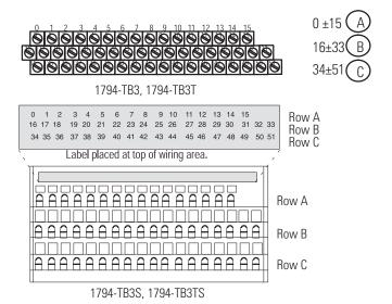
4. If daisy chaining the +24V DC power to the next base unit, connect a jumper from terminal 51 on this base unit to terminal 34 on the next base unit. Connect the 24V DC common/return from terminal 33 on this base unit to terminal 16 on the next base unit.
