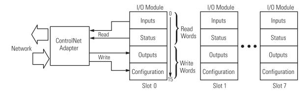
The I/O map for a module is divided into read words and write words. Read words consist of input and status words, and write words consist of output and configuration words. The number of read words or write words can be 0 or more. The length of each I/O module's read words and write words vary in size depending on module complexity. Each I/O module will support at least 1 input word or 1 output word. Status and configuration are optional, depending on the module.
