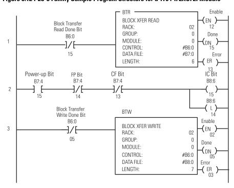
Figure 3.13 PLC-3 Family Sample Program Structure for a 1794-OF4I Module
