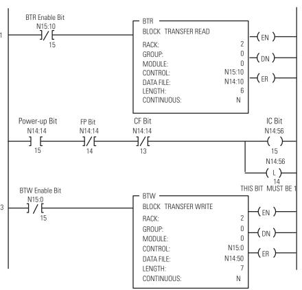
Figure 3.16 PLC-5 Family Sample Program Structure for the 1794-IF2X0F2I
