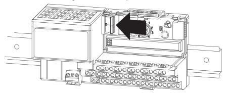
Gently push the flexbus connector into the side of the adapter to complete the backplane connection.
