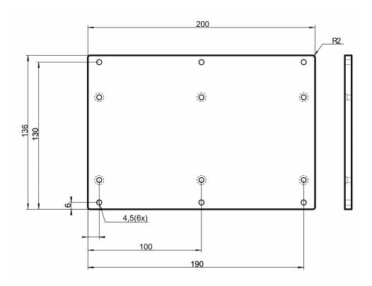
Figure 9: Aluminum Plate with Dimensions
