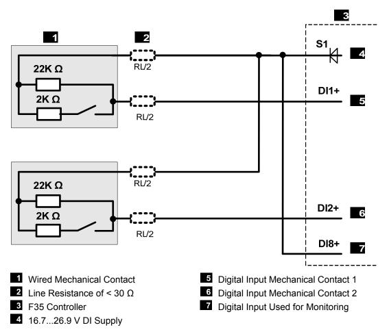
Figure 12: Wired Mechanical Contact on Digital Inputs
