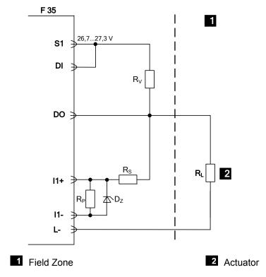
Figure 3: Circuitry for Line Monitoring
