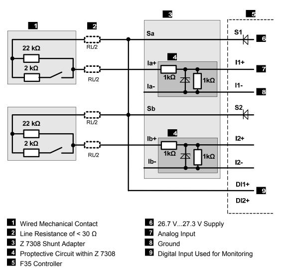
Figure 11: Wired Mechanical Contact on Analog Inputs
