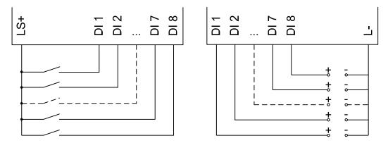
Connection of potential-free mechanical Connection of signal power sources contacts
