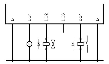
Figure 2: Connection of Actuators to Outputs
