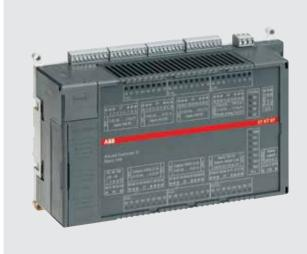
The AC31 adapter modules are based on standard AC500 I/O modules and on a specific electronic base, the modules cannot be purchased separately and are always delivered as complete devices. The pluggable electronic module cannot be replaced separately without the base.
