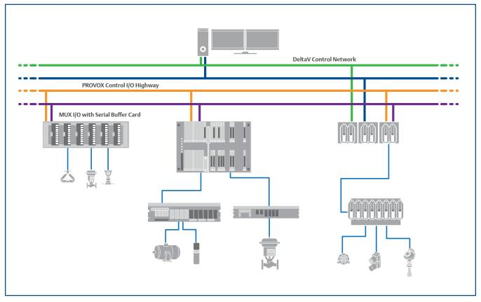
The S-Series DeltaV Controller Interface for PROVOX I/O.
