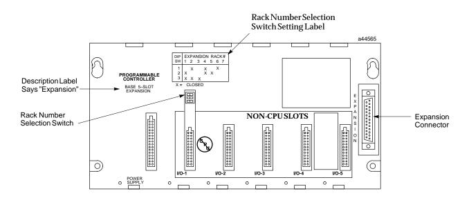
Figure 3-6. IC693CHS398 5-Slot Expansion Baseplate
