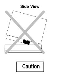
Do not tilt the Bus Interface Unit to remove it. Removing the Bus Interface Unit at an angle may cause damage.
