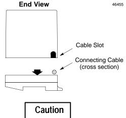
Do not exert excessive force; it may damage the equipment.
