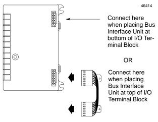
After installing the cable, be sure it is firmly seated on both connectors.
