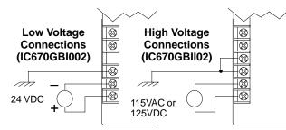
For BIU version IC670GBI102, if a DC supply is used the polarity is not important.
