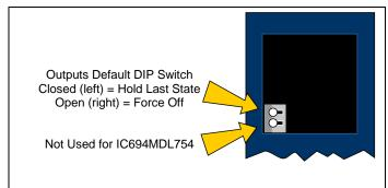
With the Outputs Default switch in the right (open) position, the outputs mode is set to Force Off. In this mode, the outputs will go to zero whenever communication with the CPU is lost. When the switch is in the left position, the Outputs Default mode is set to Hold Last State. In this mode the outputs will retain their last programmed value whenever communication with the CPU is lost, and field power is present.
