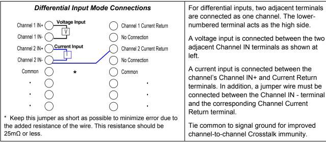
Two door cards are provided with the module: one shows connections for single-ended mode and the other shows connections for differential mode. Insert the card that matches the wiring that will be used.
