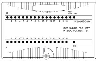
Note: Negative logic input functionality and 12V output functionality require module version -C or higher.
