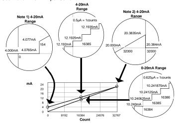
The following equations can be used to calculate count values: 4-20mA Range: Counts = ( Current in mA - 4mA) x (32000 / 16mA)
