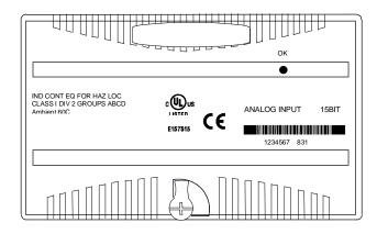
The module receives power from the backplane power supply. No external power source is required for module operation. Power for the user's transceivers must be supplied from an external source.
