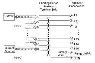
An optional Shorting Bar or Auxiliary I/O Terminal Strip can be used for wiring convenience, when multiple Return paths need to be wired together.
