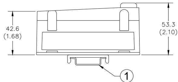
1. 35mm DIN rail DIN mount clips (when DIN rail mounting is specified)
