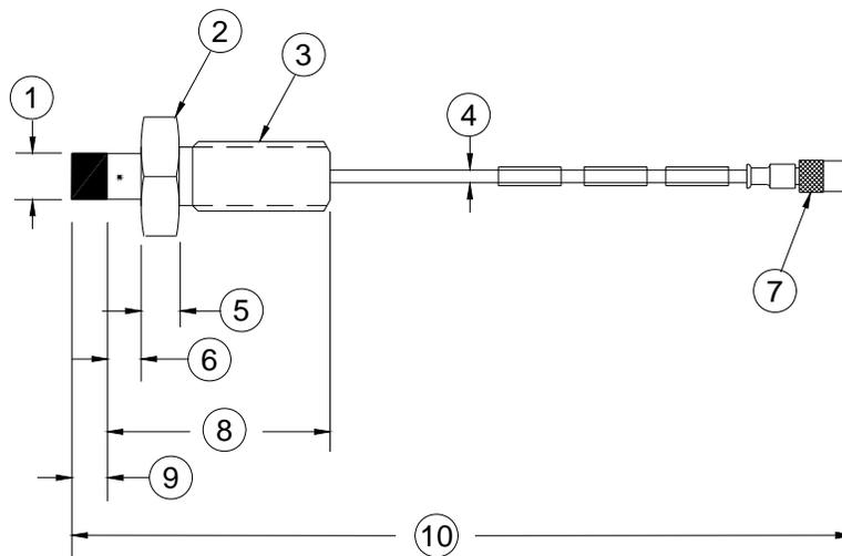
1. Probe tip, 5.26 mm (0.207 in) maximum diameter
