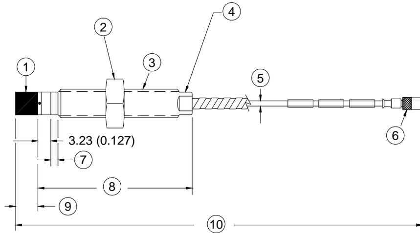
1. Probe tip, 5.26 mm (0.207 in) maximum diameter
