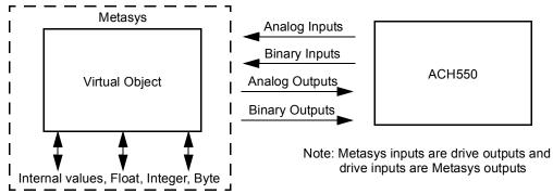
In the N2 Fieldbus protocol the ACH550 drive appears as a "virtual object".
