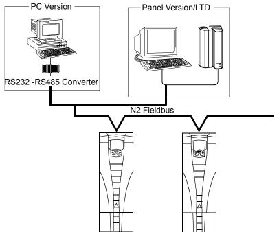
On the N2 Fieldbus each ACH550 drive can be accessed by the full complement of Metasys FMS features, including Change-of-State (COS) monitoring, alarm notification, scheduling, trend, and totalization.
