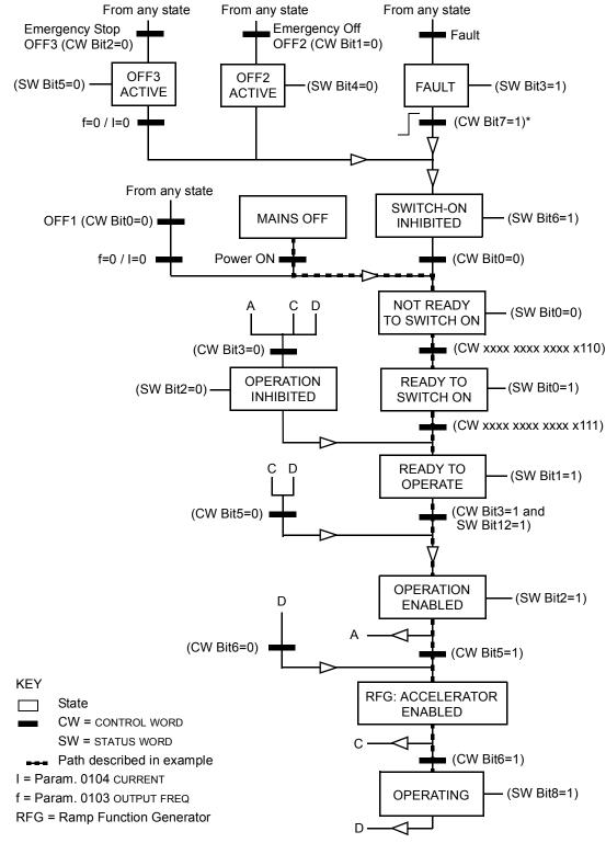
The state diagram below describes the start-stop function of CONTROL WORD (CW) and STATUS WORD (SW) bits for the ABB Drives profile.
