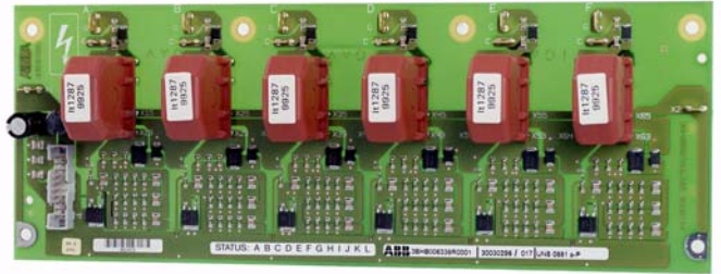
Fig. 4.2-10 Block diagram and view of Gate Driver Interface GDI
