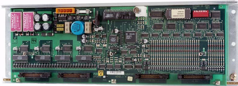
Fig. 4.2-27 View of fieldbus coupler FBC
