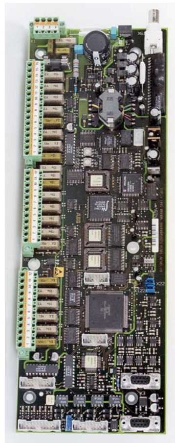
Fig. 4.2-8 Block diagram and view of converter interface CIN
