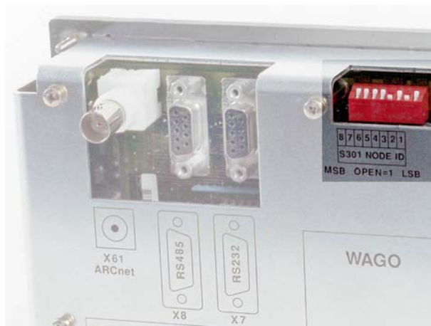
Fig. 4.2-24 Setting ARCnet node address
