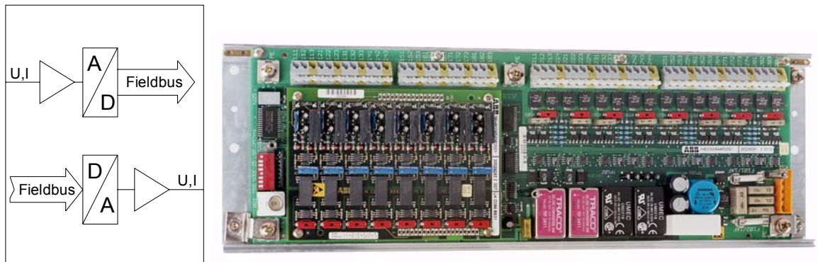
Fig. 4.2-32 Block circuit diagram and view of Analogue I/O interface AIO
